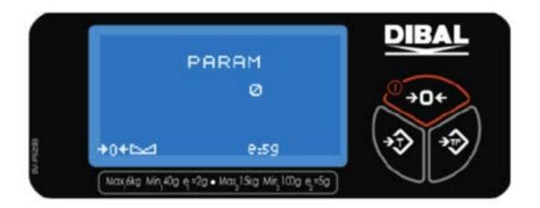
By pressing 0, you will increase the communication parameter setup, pressing T will decrease the selection. You can leave the selection at 0, which according to the following table gives you communication at 9600 baud, 8 data bits, 1 stop bit, no parity:
